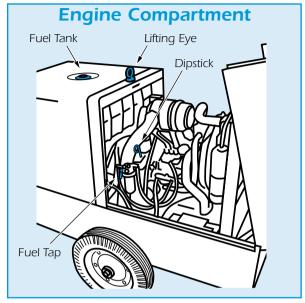
With the machine on firm level ground, open the engine compartment cover and check fuel and oil levels (see EQUIPMENT CARE).
