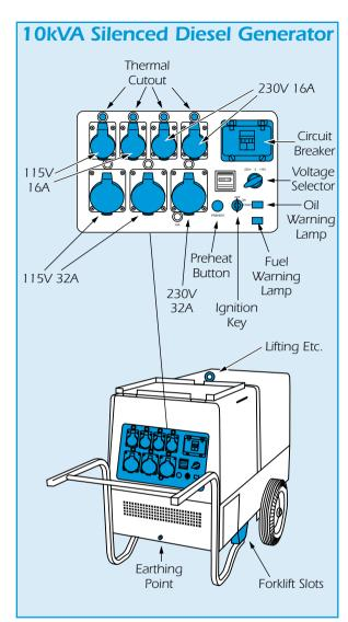
Connect up the equipment you want to power using suitable cables and plugs, making sure their switches are OFF.
