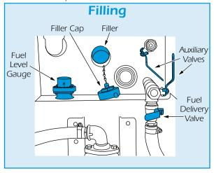
You should only fill the unit with clean diesel or **DERV**, if the diesel becomes contaminated, contact your local HSS Hire Shop for advise.
