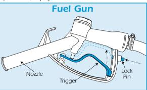
**To transfer diesel** open the rear cover and remove the fuel gun. **Insert the nozzle into the fuel tank** being filled and **lock the trigger open.**
