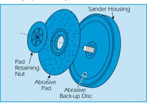
To fit a new abrasive pad (100 grit only), grasp the abrasive pad and the sander housing to prevent pad rotation.
