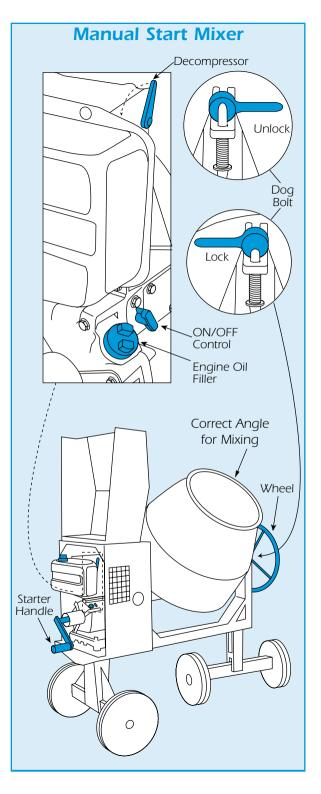
Once the mix is ready, **discharge the contents into a wheel barrow.** To **tip the drum** take a firm hold on the wheel then release the dog bolt on the drum control wheel and slowly turn the wheel to discharge its contents. Be careful, use both hands on the wheel and be prepared for the transfer of weight as the mix moves to the end of the drum.
