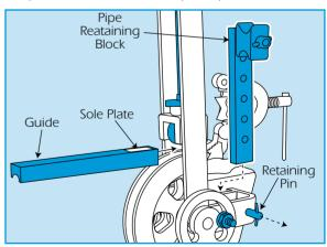
Lower the roller assembly on the quide lever, until it is either in contact with the quide, or for conduit, in direct contact with the pipe.
