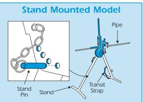
Unfasten the transit strap, remove the stand pin, set the stand on firm around, open the leas to the desired height and relocate the stand pin.
