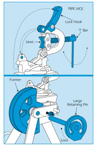
Place the correct former in position (it can't be fitted up side down!) and replace the large retaining pin. ensuring it is fully home, then lock in place by turning the pin clockwise.
