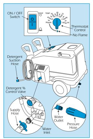
Always switch OFF the equipment when not in use. The burners exhaust get very hot so keep your distance. Never look directly into the exhaust port nor cover it at any time.
