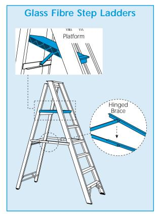
The steps are designed to provide access for light maintenance work. Never use them as a work platform.
