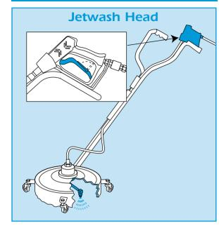
Set the engines throttle control to 'fast', release the trigger lock then squeeze the trigger to begin work.
