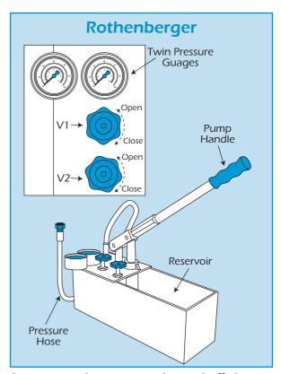
Any pressure loss can now be read off the test pressure gauge. Where 2 gauges are fitted both must read the same pressure, if not, stop and contact your local HSS Hire for advice.
