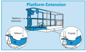
awkward areas. To deploy the extension, **depress the platform extension release pedal with your foot and push the platform extension with the guardrail.**
