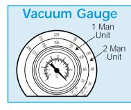
ready for lifting. Observe the reading on the vacuum gauge, the two outer scales will help you d e t e r m i n e whether the lifter has a sufficient hold on the slab in comparison to its weight.
