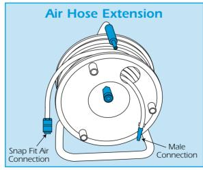
Next, connect a pressure air hose between the air outlet on the pot and the air inlet on the spray guns handle or side entry (Multi-Flek).
