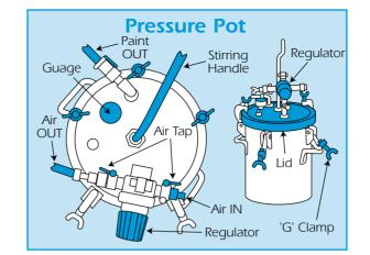
Release and swing the 'G' clamps clear of the pots lid. Lift the lid clear and place upside down on a clean surface.
