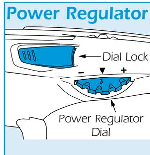
Start at the number 1 setting, make a test fixing (see Basic Techniques) then reset the regulator dial if required and re-test until you have an acceptable fixing.
