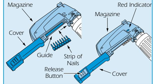
hear a click as the fastener guide slides back and arms the firing mechanism.
