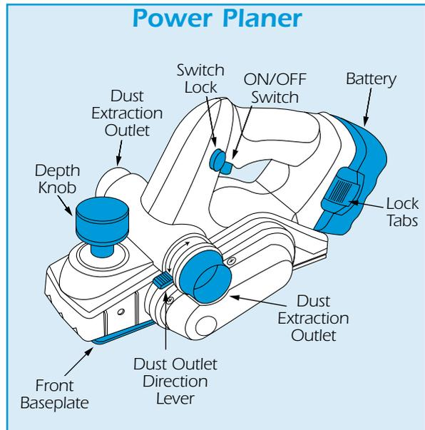
The power planer is fitted with an ON/OFF switch lock, which prevents accidental operation of the unit. The spring loaded lock is manually operated and must be moved either to the left or right to release the ON/OFF switch.
