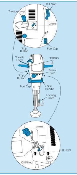
the engine stops after a short time this may be due to vapour lock, to rectify this: close the choke by turning the control upward, depress the throttle lever to full speed position and pull the starter cord.
