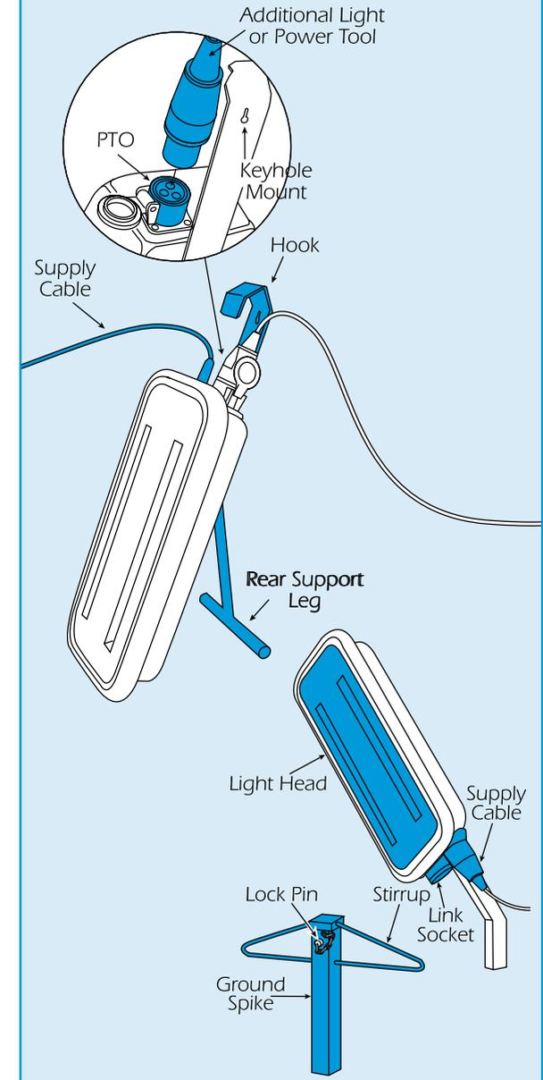
Then push the spike into the ground (checking all the time that the spike is vertical) until the stirrups are level with the ground.
