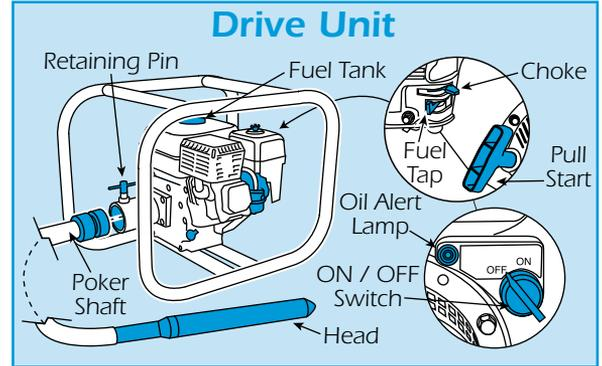
The throttle is fixed in the 'fast' position and MUST NOT be altered or tampered with, as the engine is set to the correct RPM for the poker head. Two or three pulls on the starter cord should start the engine.
