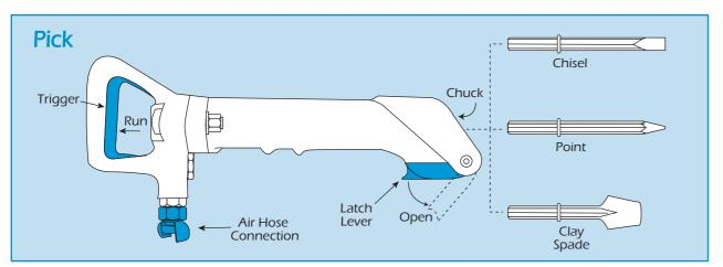
If the steel becomes jammed in the work DO NOT use the breaker/pick as a lever. Tease the steel from the work by pushing then pulling.
