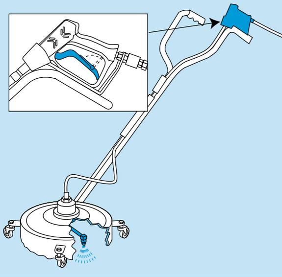
Release the trigger lock on the lance then squeeze the trigger to begin work.
