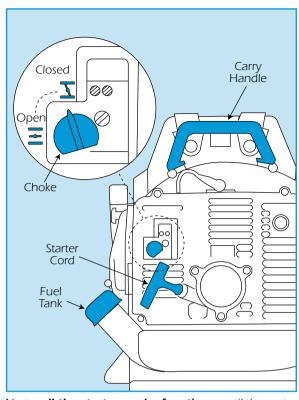
Next pull the starter cord a few times until the motor 'coughs', fully open the choke and pull the starter cord once more. The motor should start.
