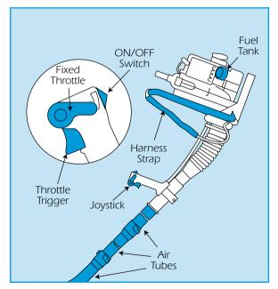
The fixed throttle control allows you to set the engine speed without having to hold the throttle trigger. The control can be set between idle and full throttle. If you wish to use the normal throttle trigger set the fixed throttle control at its lowest position (see illustration).
