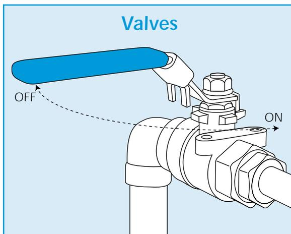
Open both flow valves and switch the pump ON. Make sure that the liquid level in the tank remains above the minimum mark as more water may need to be added.
