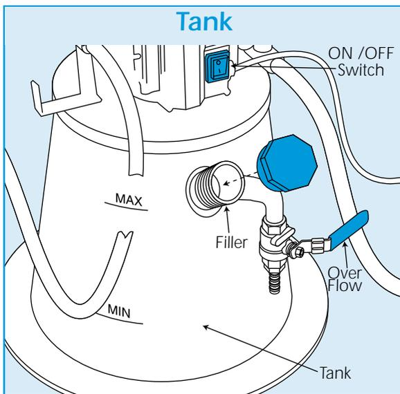
Fill the unit with the appropriate amount of flushing chemical and top up with fresh clean water to approximately 150mm below the maximum liquid level.
