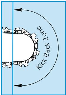
**Never let the chain touch the ground, nor any metal or masonry obstructions. This will cause 'kick back' and will damage the blade.**
