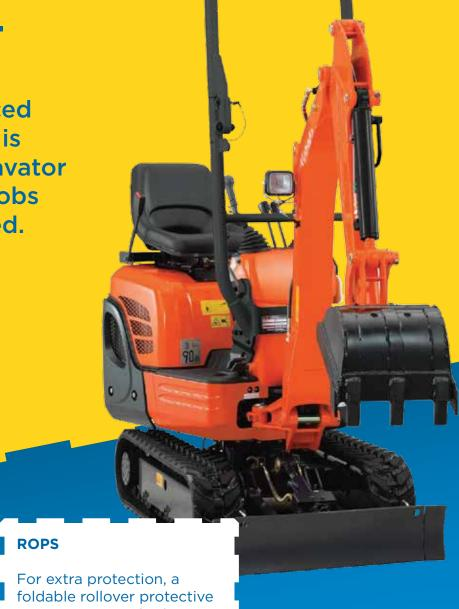
structure is standardequipped on the K008-3.
