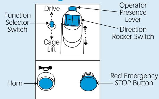
Turn the ground control selector key to the 'cage' position and check that the red emergency STOP button is pulled out to the ON position.
