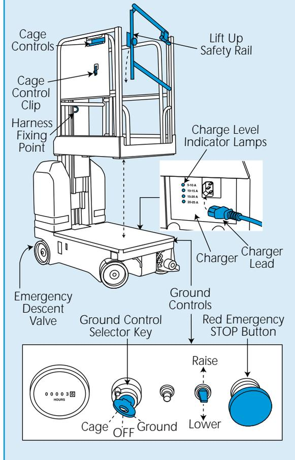
Turn the ground control selector key to the 'ground' position and check that the red emergency STOP button is pulled out to the ON position.
