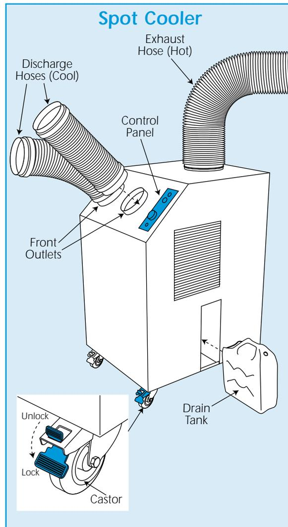
If the temperature in the room is above 35°C, reduce the temperature by opening all doors/windows and operating the unit's fan (without cooling), to circulate the air.
