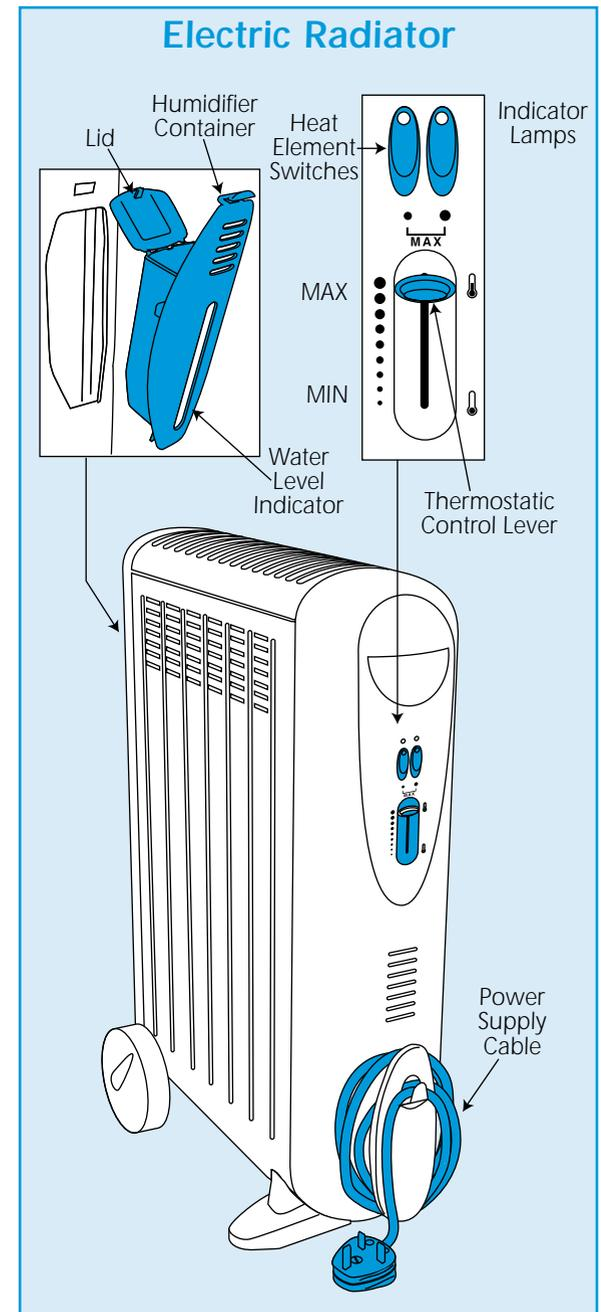
Once the room has reached the required heat, move the thermostatic control lever down until the heater switch indicator lamps go out.
