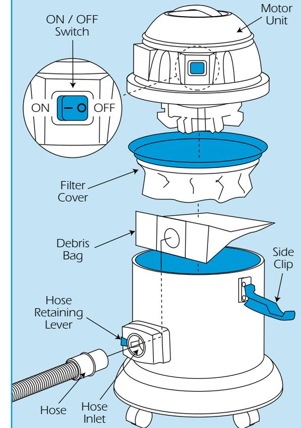
**To switch the vacuum ON** simply **move the ON/OFF switch to the 'I' position.** To switch OFF move the switch to the 'O' position.
