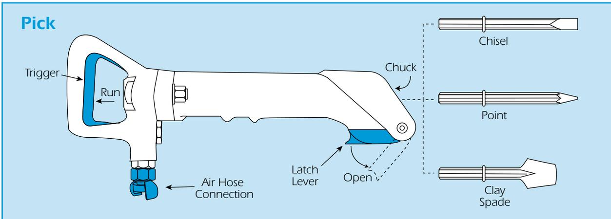
Lift it clear before turning OFF, and wait for moving parts to stop before putting it aside.
