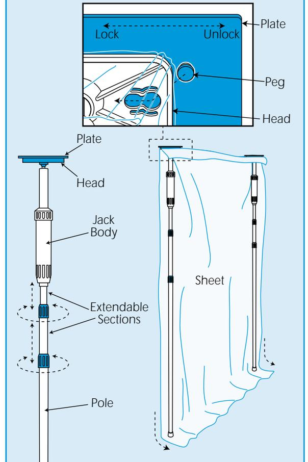
Lock the plate to the head by sliding the plate forward.
