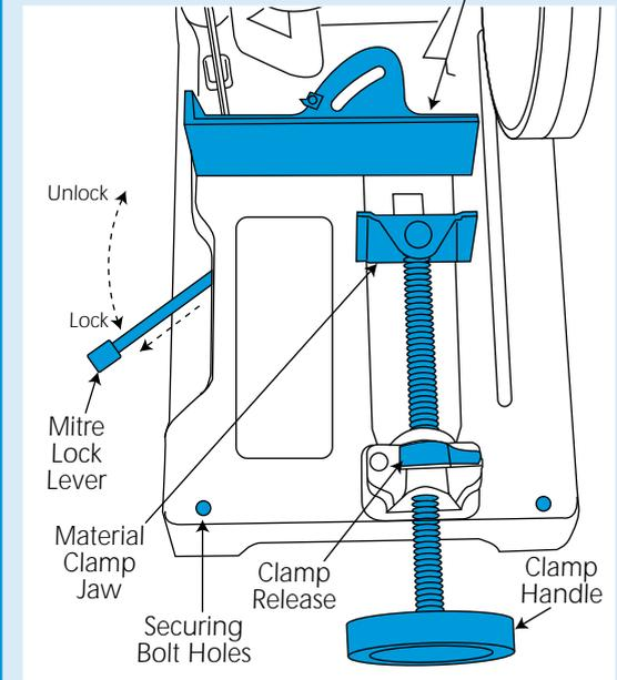
Turn the clamp release and pull the clamp assembly fully back. Place the material against the rear fence and push the clamp assembly forward until it is in contact with the work piece.
