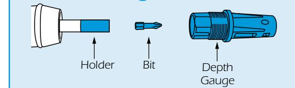
Fit the machine with right bit for the job.
