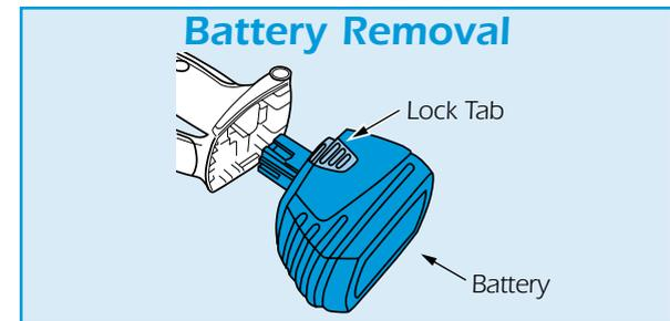
Fit the battery to the Drywall Screwdriver, simply push into the base of the handle until it clicks into position.
