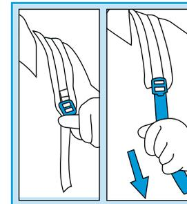
Lift the machine up and place the harness straps on your shoulder, pull the ends of the straps down to tighten then adjusting as necessary for comfort.
