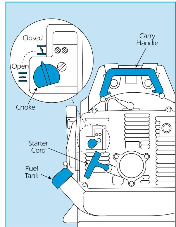
Next pull the starter cord a few times until the motor 'coughs', fully open the choke and pull the starter cord once more. The motor should start.
