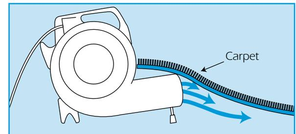
**The angle of the outlet can be adjusted** to suit the application, **to raise the outlet, screw the front legs out, to lower screw the legs in.**
