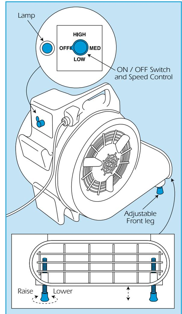
**Lift the edge of the carpet and place the fan's outlet under the edge** inserting as far as it will go.
