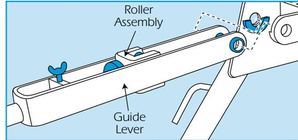
Lower the guide lever then take a firm hold of the fitted former and withdraw the large retaining pin followed by the former.
