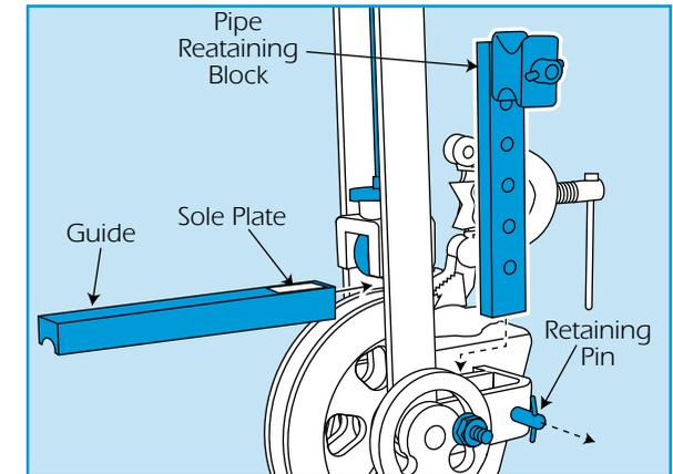
Lower the roller assembly on the guide lever, until it is either in contact with the guide, or for conduit, in direct contact with the pipe.
