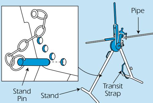
Unfasten the transit strap, remove the stand pin, set the stand on firm ground, open the legs to the desired height and relocate the stand pin.
