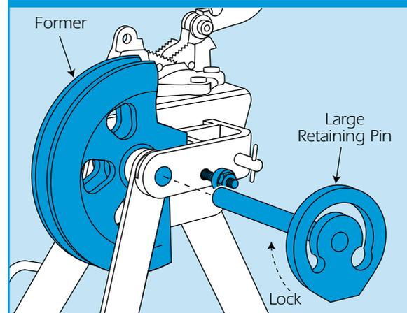
Place the correct former in position (it can't be fitted up side down!) and replace the large retaining pin, ensuring it is fully home, then lock in place by turning the pin clockwise.
