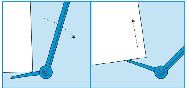
**The crowbar must not be steered with the load stationary,** steering may only occur when the load is moving.
