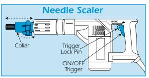
with a suitable 110v generated supply, or powered from the mains via a suitable 110v transformer (minimum 2.2kva tool rating).
