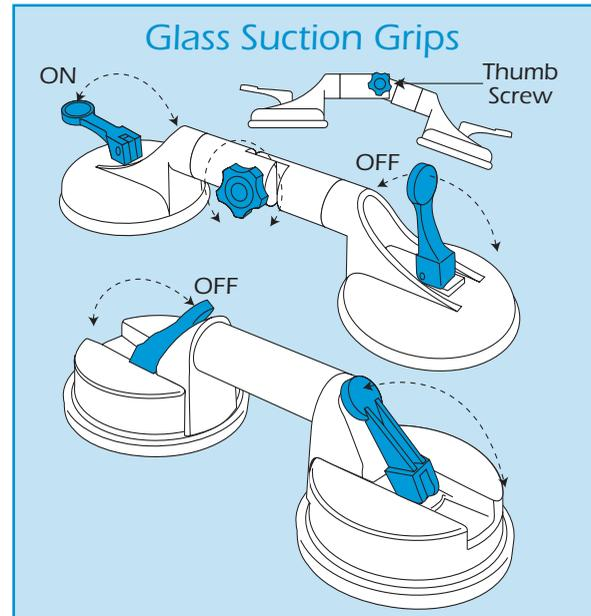
press the cup faces against the glass surface, then fully push the suction levers down, one at a time, to create the vacuum grip.
