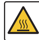
Danger Hot exhaust
