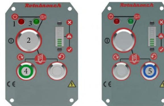
1. Ensure power to the machine, red LED will illuminate (1).
