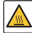
Danger Hot exhaust
