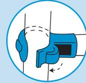
**LOCKING CLAWS** join braces to frames. Pull back the trigger to open the jaws, then snap the claw onto the rail or upright, ensuring the open side faces down or out. The jaws should lock automatically.
