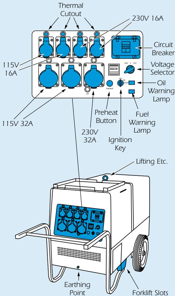
Connect up the equipment you want to power using suitable cables and plugs, **making sure their switches are OFF.**
