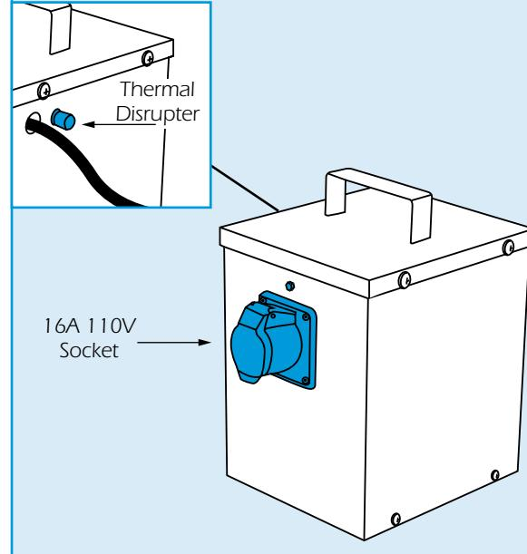
**Position the transformer in a safe place,** as close to its power supply as possible.
