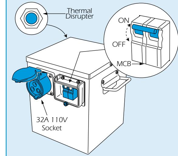
If tool rated, you can power equipment up to its total rate for a maximum of 30 minutes, after which the transformer will need to cool. If you continue to use it at full rate, the internal coils will overheat and the transformer may be permanently damaged.
