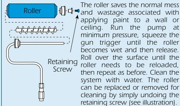
The roller saves the normal mess and wastage associated with applying paint to a wall or ceiling. Run the pump at minimum pressure, squeeze the gun trigger until the roller becomes wet and then release. Roll over the surface until the roller needs to be reloaded, then repeat as before. Clean the system with water. The roller can be replaced or removed for cleaning by simply undoing the retaining screw (see illustration).
