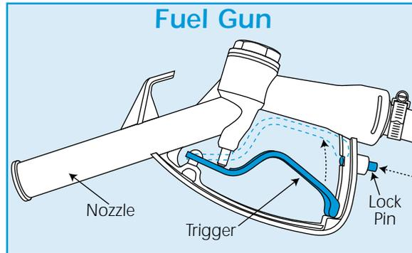
To transfer diesel begin by removing the gun from its holster, place the nozzle into the container being filled and lock the trigger open.
