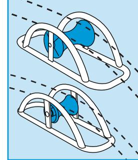
Once all necessary adjustments have been made, roll the cable drum onto the rollers ensuring the cable feeds off from the bottom of the drum and not the top.
