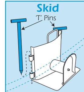
When setting the rollers out, make sure that they are set in a straight line, or the cable will fall off the roller.
