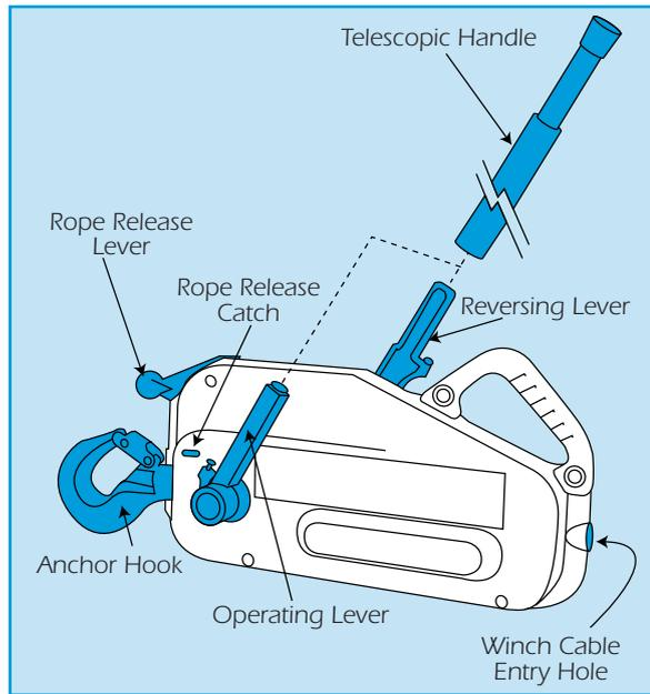
When you are ready to lower (or release) the load, place the telescopic handle onto the reversing lever and again crank the handle back and forth. The cable will be drawn out on each forward stroke.
